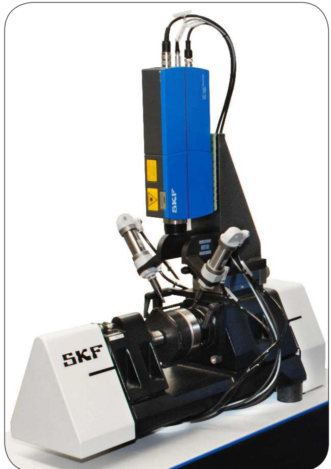
MVH 90EL mechanics with axial and radial load
