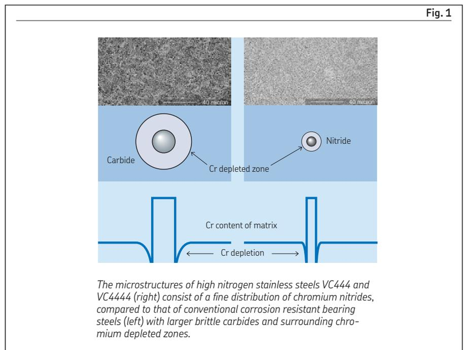
gen stainless steel VC4444 has slightly less corrosion resistance but otherwise similar properties and is suitable for operating temperature ranges from very low (cryogenic) to very high.
